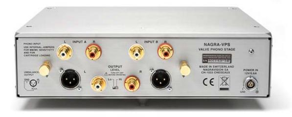
outputs, along with a grounding post. There is also a pair of XLR's, but this is not a fully balanced device, so there is no major advantage to using the balanced outputs. An umbilical cord goes from the VPS to the same ACPS II power supply that powers the Nagra PL-L linestage or their CDP CD player.
